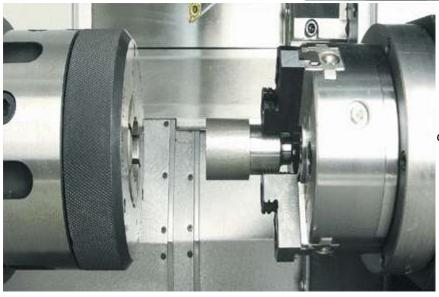
The Tornado T6MS and T8MS 5 Axis CNC Lathes are true 'Single-hit' turning centers. The addition of a powerful sub spindle, controlled from the state-of-the-art G.E. Fanuc 18i TB control, allows 5 axis programming. 'MS' models have all the machine design features of the 2 & 3 axis models but with the added production flexibility of a sub-spindle and live tooling.
