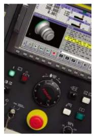
Two and three axis Tornado models are fitted with the GE Fanuc 21iTB control while the five and six axis 'MS & MSY' models are fitted with the 18iTB control. These ultra-compact controls from the world's leading CNC supplier are all digital with twice the processing speed of the previous 'A' model controls and incorporate the latest Manual Guide i as standard.
